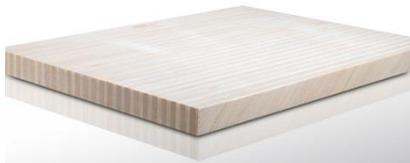
**BALTEK® VBC** is an engineered core material produced from certified, kiln-dried and oriented balsa wood layers. Its unique mechanical properties and process ability are obtained by the optimal alignment of various layers. **BALTEK® VBC** is an ideal, sustainable core material made of renewable resources with a very broad range of use.
