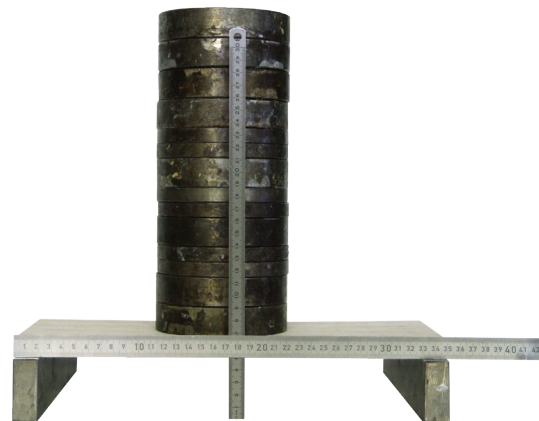
Figure 4: Deflection of BALTEK® VBC core lengthwise load.
