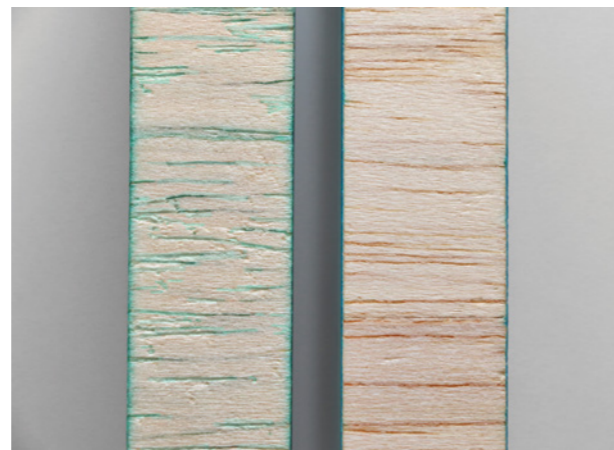
Visualization of resin uptake in cross section of infused balsa wood. Left: resin filled vessels in standard balsa. Right: BALTEK® SealX .
