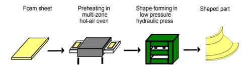
In a first step, the foam sheets are preheated to the required temperature. This operation should be long enough to reach the desired temperature in the centre of the core. The metal tool for shape-forming should be temperature controlled. The mould can be opened only after the core has reached a temperature below Tg also in the centre.
