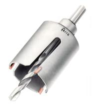
Plugs or large diameter holes can be cut-out even from higher density foam sheets with the help of special cutter cylinders. The numbers of bits are preferably kept low (for example about four). The use of hard-point tools is recommended. The cutting speed and feed-rate depends on the material characteristics and is best ascertained individually.
