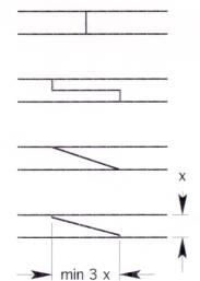
There are several ways butt joints of foam sheets can be made. Depending on the thickness of the foam and the desired properties of the final part, one or the other geometry is suitable. In general, it should be kept in mind that the area of the joint should be big enough. Some possibilities are shown in the pictures on the left. Recommendations for adhesives to be used can be found in **chapter 2.5**
