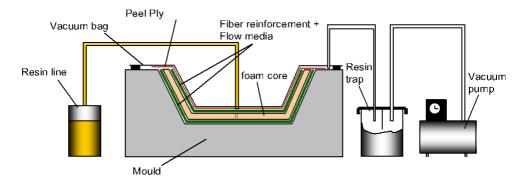
The disadvantage of flow mats is that resin rich skins are produced. The fibre content is reduced to 20% or even less in these layers.
