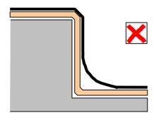
Chamfering the foam provides smooth transitions between single skins and sandwich or between different core thicknesses.
