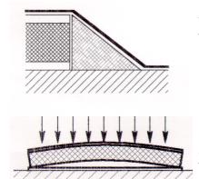
The upper edges and corners of sandwich panels, especially those with thicker low density foam cores should be protected from localized stress by framing the panel with wedges of suitable dimensions made of wood or plastic foam.
